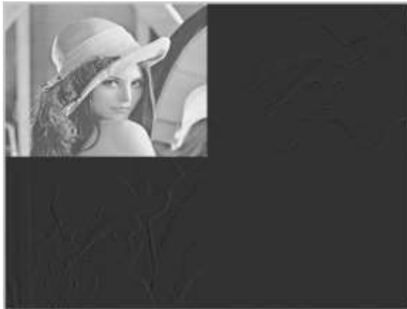
Fig. 2. LL, LH, HL and HH subbands of Lena's image obtained by using DWT.
